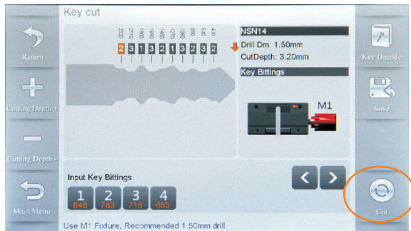
4) Put the new blank key to the correct position and click on 'Cut' for cutting keys.
