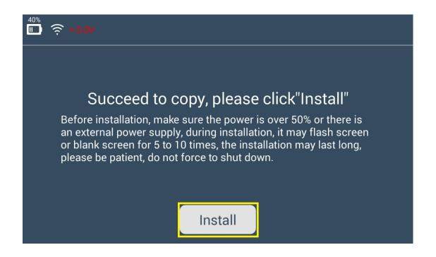
5. Blank screen is normal during the installation. The whole process will take 5 minutes, be patient to wait and don't restart the device manually.
