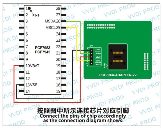
Note: If PCF79XX adapter option can't recognize chip due to the affection of circuit board, just remove chip and put it in IC socket, then use option "PCF79XX chip" to operate.
