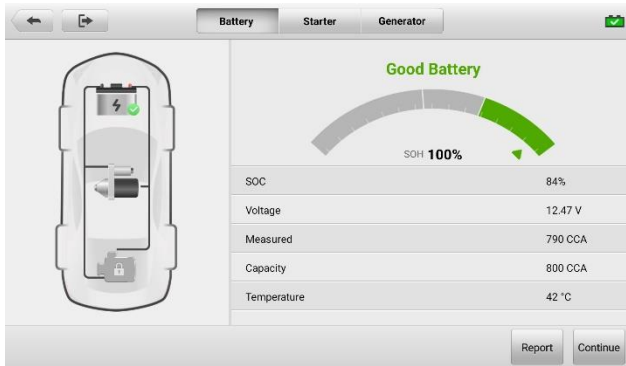
Figure 6-7 Sample Battery Test Results Screen
